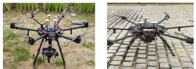
Figure 5: Small category drone with Hyperspectral camera (L) & Lidar (R)
